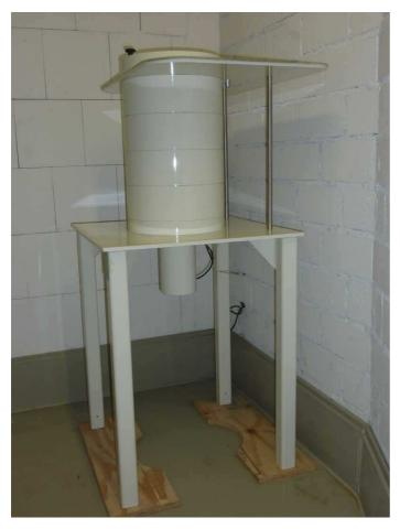
Background radiation is suppressed through a lead shield having thickness of 50 mm or more of very low-activity lead. The inner space of the lead castle is sufficient for a 1-liter Marinelli beaker or up to 2-liter standard beakers. An optimised sample geometry, i.e. highest count-rate, is achieved with a 1-Liter Marinelli beaker.
