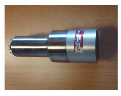
3"x3" Nal(Tl) detector with integrated photomultiplier and very strong μ-metal shield (0.63 thick) against external magnetic fields. All components are hermetically sealed in aluminium housing (optional SS housing). The Al-thickness around the detector crystal is 0.5 mm; the inner reflector layer consists of Teflon.
