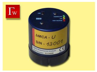
Multichannel analyzer (MCA) model "bMCA" with HV-generator, Amplifier/Shaper, flash-ADC and up to 4k (4096 channels) spectrum length.
