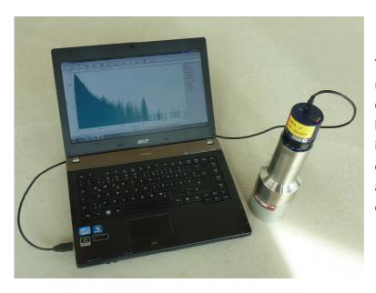
The basic operating unit for the multichannel analyzer consists of a desktop PC with monitor, keyboard and mouse or, as shown in the picture, of a Notebook. An optional Laser Printer can be attached for immediate documentation.
