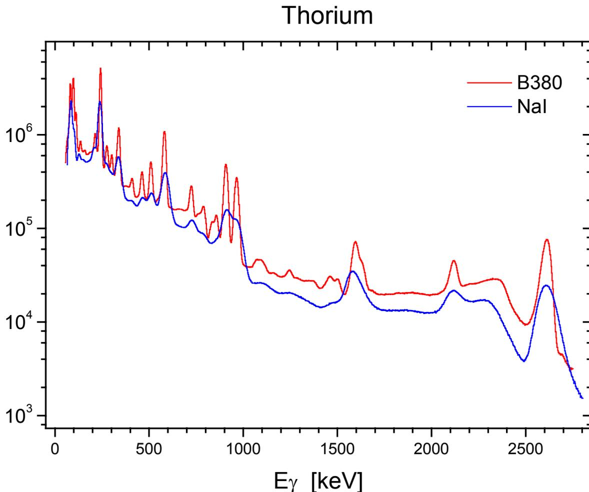
**Figure 1:** Spectra measured under identical conditions with a NaI(Tl) and a BrillanCe detector from a Thorium source.
