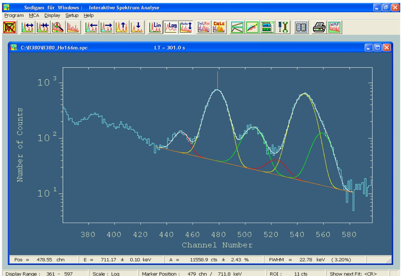
Figure 4: Fraction of a  $^{166m}\text{Ho}$  spectrum together with multiplet fit display.
