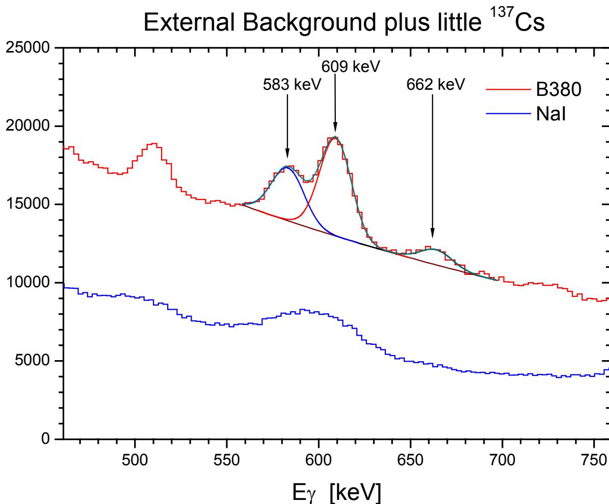
**Figure 2:** Section of ambient background spectra measured with BrilLanCe and NaI(Tl) detectors under identical conditions. Full lines in the red spectrum are the baseline, fitted peaks and the sum function.
