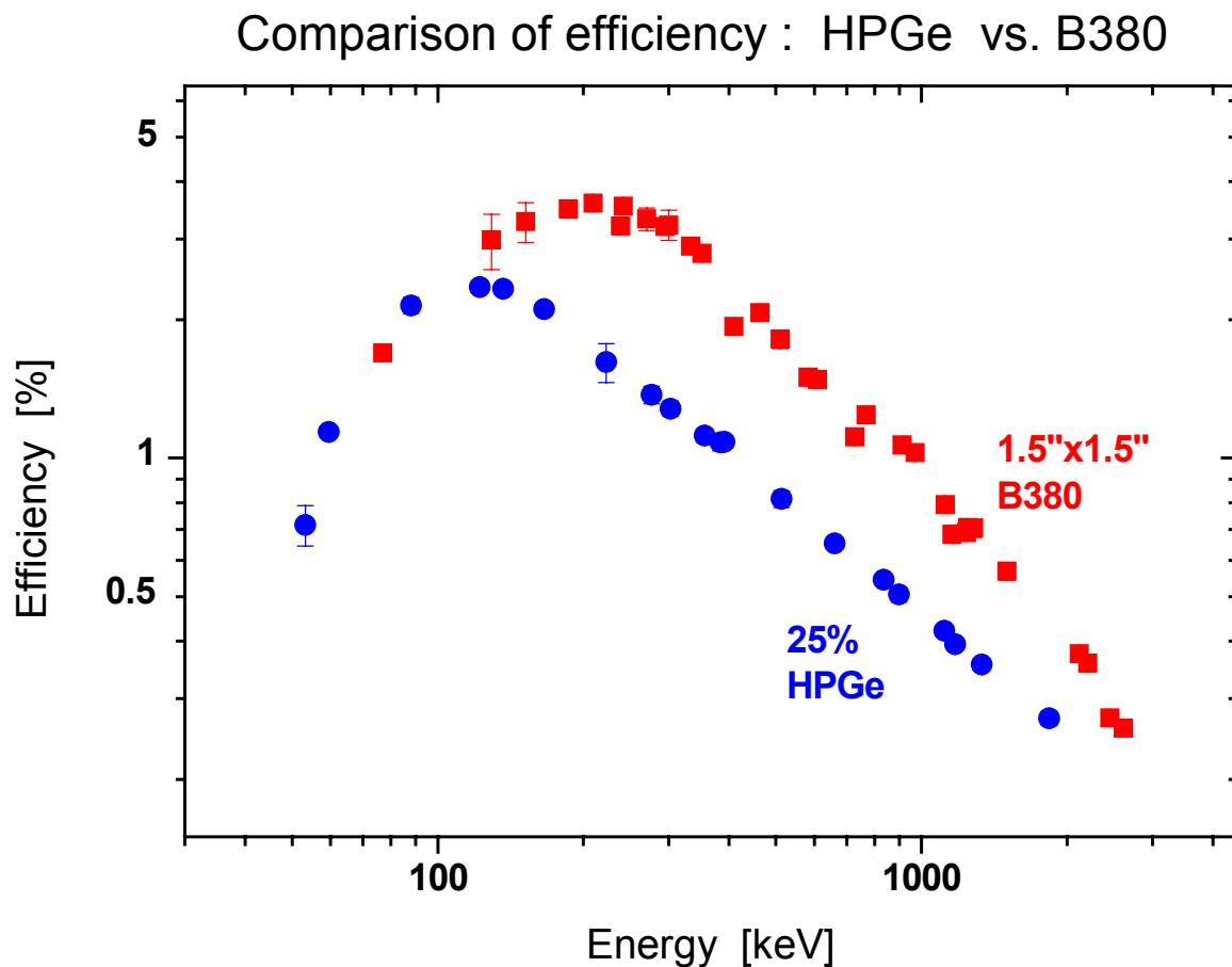
*Figure 3:* Full energy peak efficiency functions for a 25% (rel.) p-type HPGe and a 1.5''x1.5'' B380 detector.
