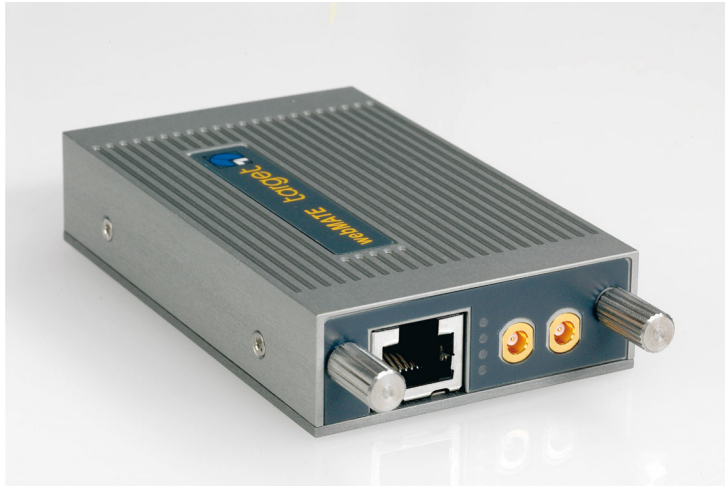
Figure 1: Example of an Ethernet- based 64k MCA that can be directly connected to any commercial ADC
