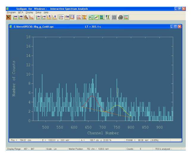
Spectrum measured for 5 minutes with a 3"x3" NaI(Tl) detector inside a 50 mm thick lead castle from 100 grams sample containg 0.10~Bq/g of  $^{60}Co$ . The spectrum was measured with a detector having 7% resolution (FWHM for the 661.6 keV peak from  $^{137}Cs$ )
