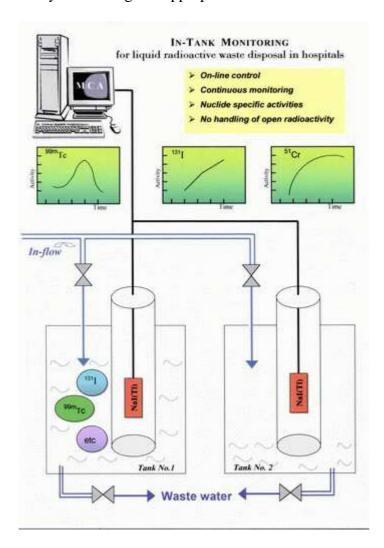
In modern systems, handling of open radioactivity samples is no longer necessary. A medium size 2"x2" NaI(Tl) detector is mounted inside each of a facility's sewage tanks in a submerged watertight tubing. The detector sits almost at the bottom of the tank. A multichannel analyser with SODIGAM software selects which tank/detector is to be measured and controls all data manipulations.
