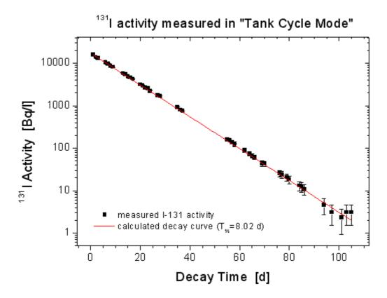
The automatic surveillance of several decay tanks in cyclic mode (see example below) will provide at least one data point per day for the decay curve as shown in the graph and per container. Spectra are analysed with SODIGAM yielding reliable activity results over many orders of magnitude, the lowest being fairly below the German "Freigabe-Grenzwert" (the legal limit of radioactivity for release to the sewage system) of <5 Bq/l.
