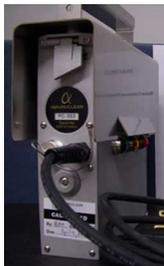
The same principle of measuring spectra from deposited progeny is applied in the continuous working level monitor PRISM 595 which is designed for personal monitoring in mines, caves, waterworks and other locations where Rn-dosimetry is an issue. The sturdy 8"x8"x2" unit contains batteries for 8 hours of operation, pump and electronics and it can be carried by a handle.
