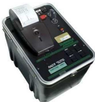
The RAD-7 spectrometer and pump serves the same purpose, and it is also equipped with a printer for immediate documentation.
