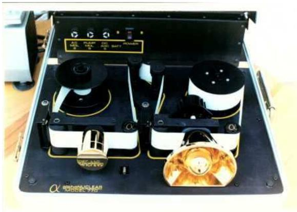
one sees the white filter tape which is moved from the supply roll (right) to the take-up roll. A controlled flow of air is sucked by an external pump via the golden funnel and through the tape where all dust particles and aerosols are deposited together with the adhering atoms of radon progeny.
